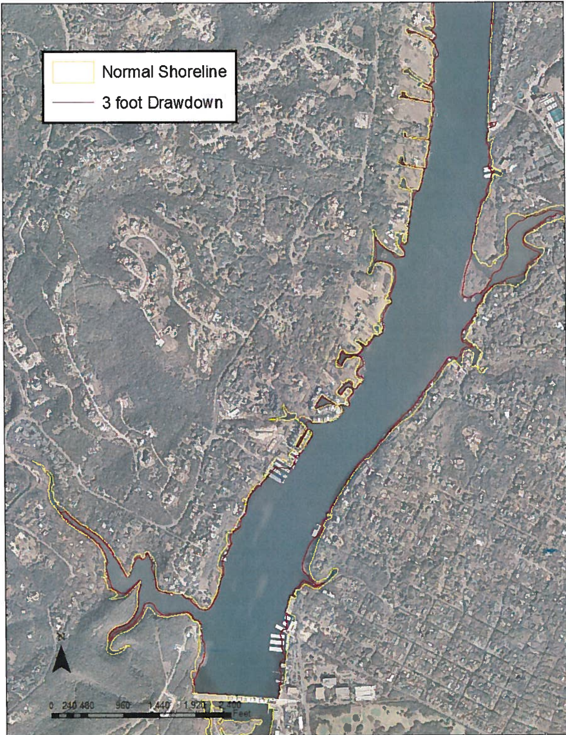
Figure 1. Downstream Lake Austin near Tom Miller Dam showing approximate location of normal water surface elevation (492.8 ft msl) (yellow) and a 3 foot drawdown (red) proposed for water supply augmentation.
