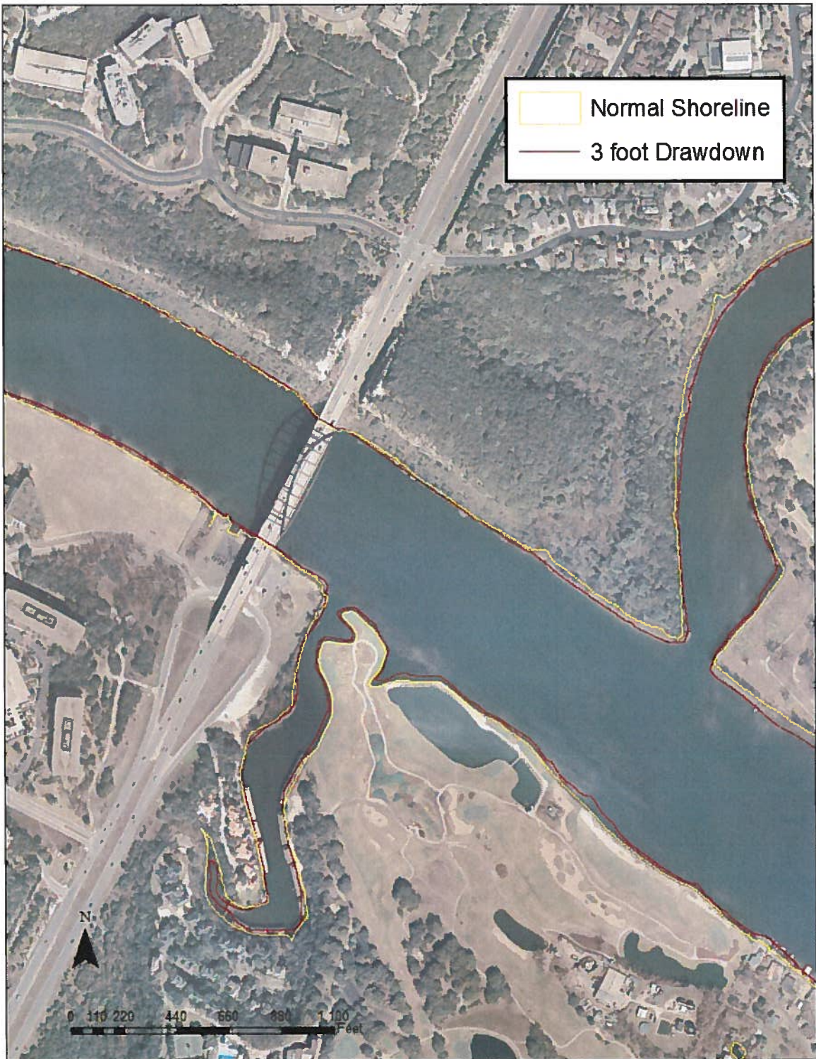
Figure 2. Lake Austin mid-reach near Loop 360 bridge and Bull Creek Cove showing approximate location of normal water surface elevation (492.8 ft msl) (yellow) and a 3 foot drawdown (red) proposed for water supply augmentation.
