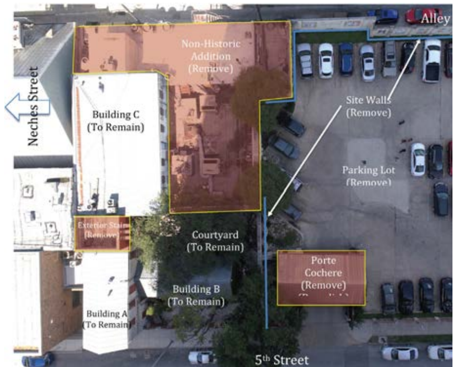
Plans indicate that demolition is being considered for non-historic buildings at the site. (O'Connell Architecture)
