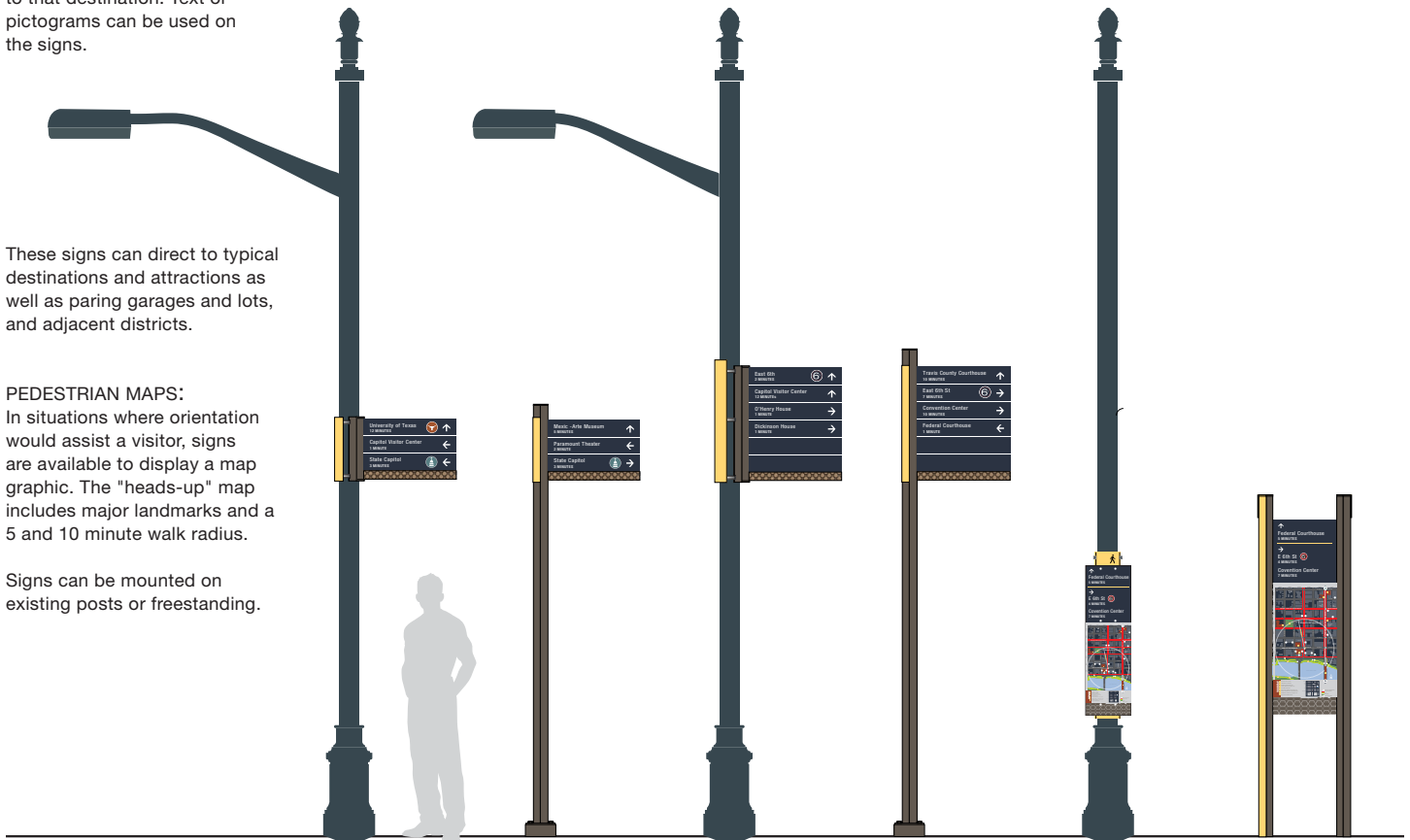
PDIR.3 PDIR.3A PDIR.6 PDIR.6A PMAP.1 PMAP.2 Pedestrian Directional Pedestrian Directional Pedestrian Directional Pedestrian Directional Pedestrian Map Pedestrian Map Utility Pole Attachment NEW POST Utility Pole NEW POST Single-Sided Utility Pole Attachment Double-Sided 2 Posts 3 messages 3 messages 6 messages 6 messages
