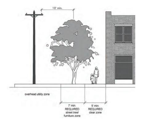
Figure 3-14: TOD Pedestrian Priority Street with overhead utilities at curb.
