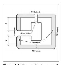
**Figure 6-1:** The net frontage length for this property is the total of lengths A and B. Required streets, drive aisles, and perimeter sidewalks are not included.
