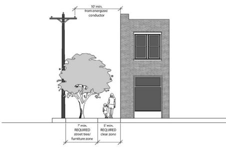
Figure 3-18: Above-Ground Utilities on TOD Local Street with utility compatible tree
