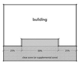
**Figure 4-5:** Sample illustrations meeting the net frontage building length requirement along a TOD Pedestrian Priority Street (no parking allowed in hatched area).
