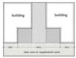
**Figure 4-6:** Sample illustrations meeting the net frontage building requirement along a TOD Local Street (no parking allowed in hatched area).
