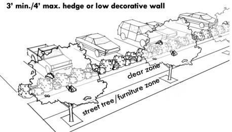
Figure 4-14: Required screening for surface parking along all streets.
