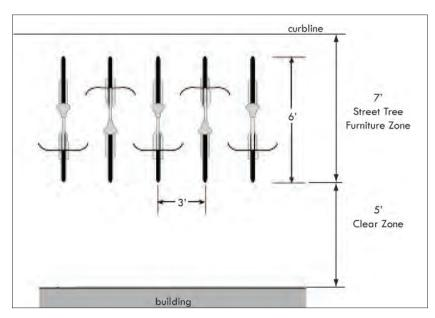
Figure 4-15: Bicycle parking design – Pedestrian Priority Street sidewalk
