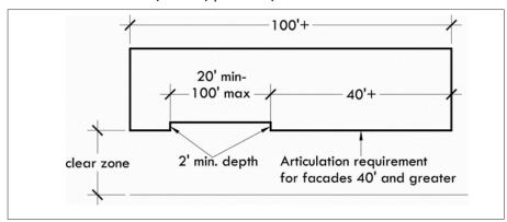
Figure 5-4: Illustration showing building façade articulation requirements
