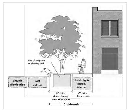
Figure 3-8: TOD Core Transit Corridor with underground utilities.
