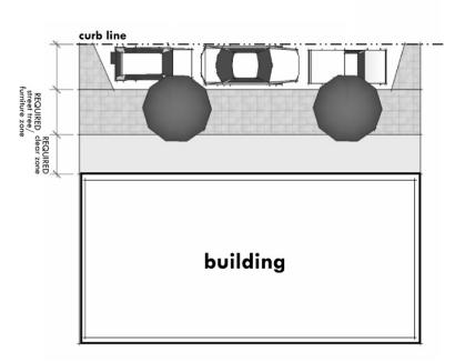
**Figure 3-20:** On-street parallel parking options; standard design (above) or a design inside the curb line (below).
